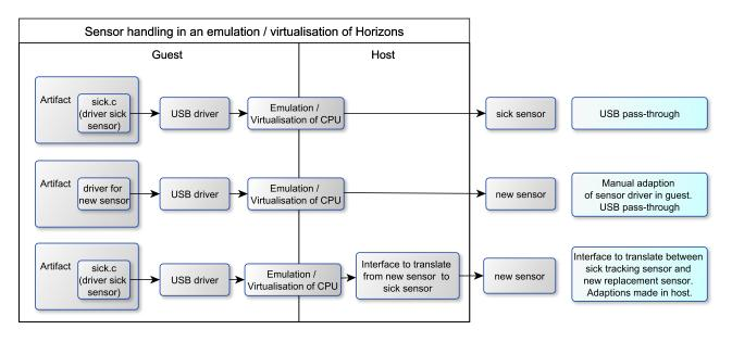
Figure 6: Emulation options for the tracking sensor of Horizons
