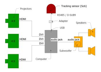
Figure 2: Equipment schematic for *Horizons* by Geert Mul (artwork creation 2008, version 2013)
