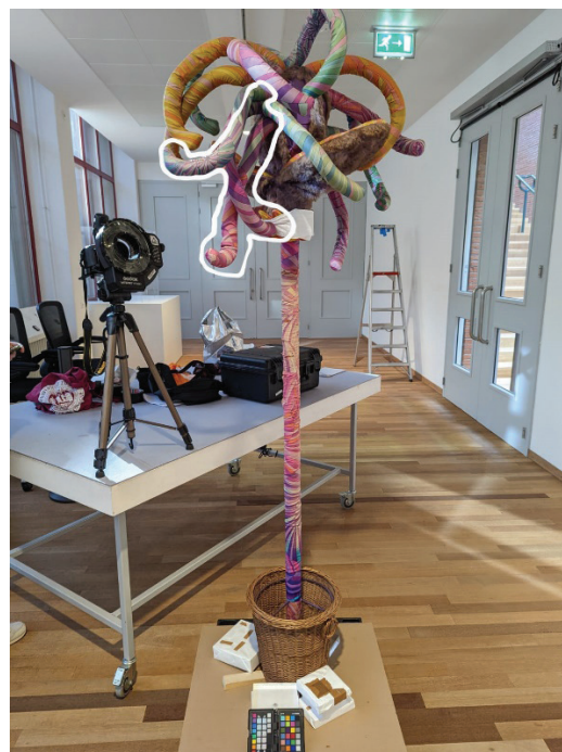
Figure 4. Setup for documentation of the colour with cross-polarised photography. Highlighted areas of tentacles used for colour matching (image by authors)..
