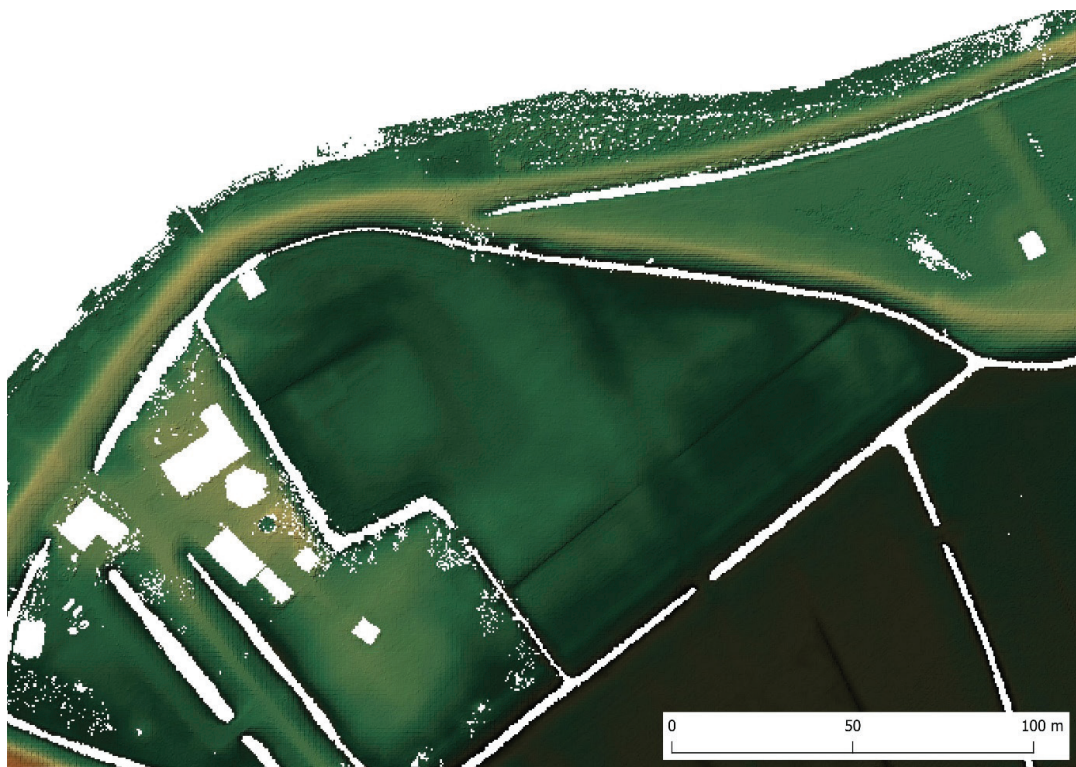
Figure 7. AHN3 data, 0.5 m digital terrain model, here visualized fused with a hillshade model.
